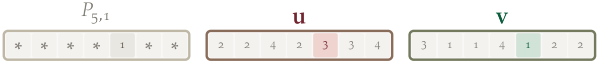
Figure 1: A Hypercube Set System . The set P_{5,1} contains all vectors with 1 at fifth position, so \mathbf{u} \notin P_{5,1} but \mathbf{v} \in P_{5,1} .
